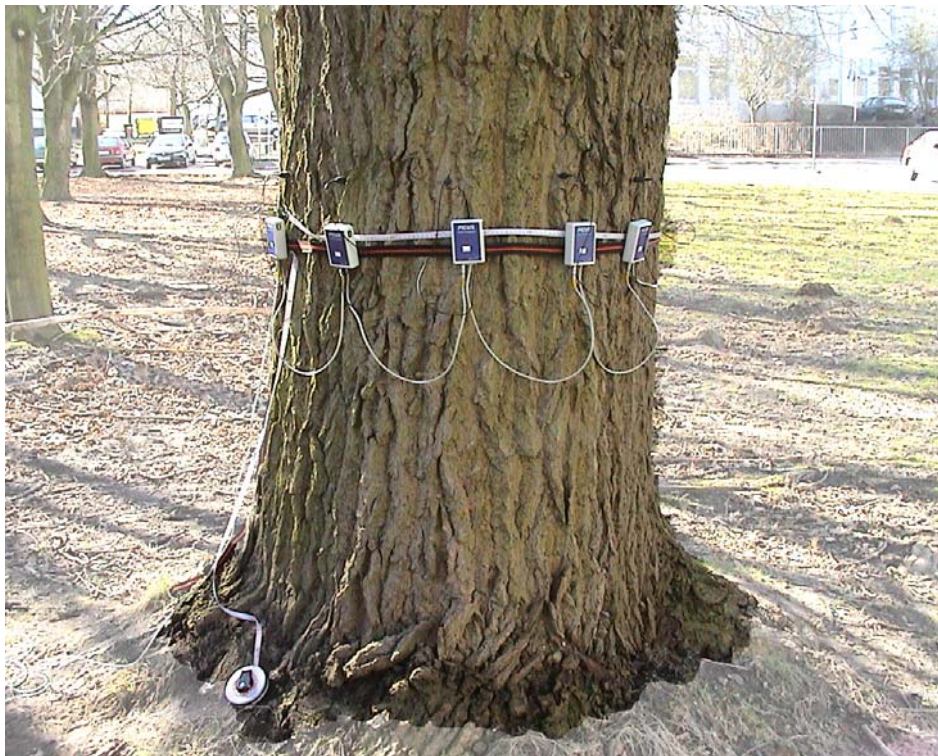
PICUS® Sonic Tomograph installed on a tree.
